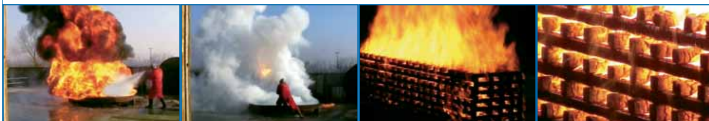
Fire test on class 233B ( 155 lts of heptane ) with a 6 kg powder fire extinguisher
